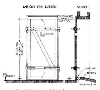
Figure 5: Gastight air raid shelter door drawing
